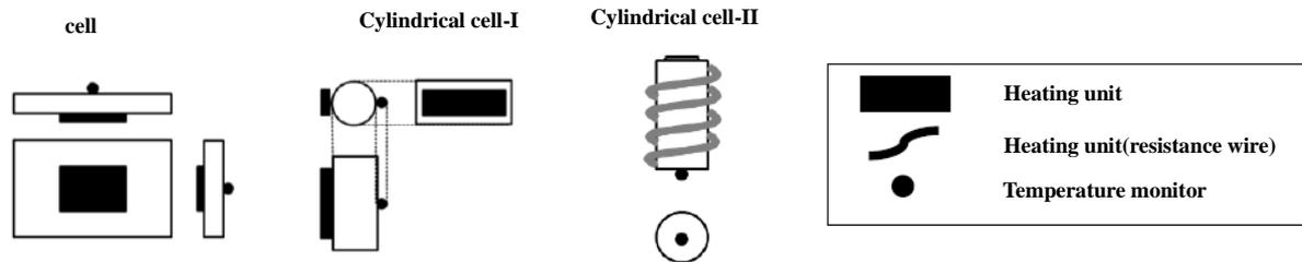
Fig. 7 Diagram of thermal runaway test
