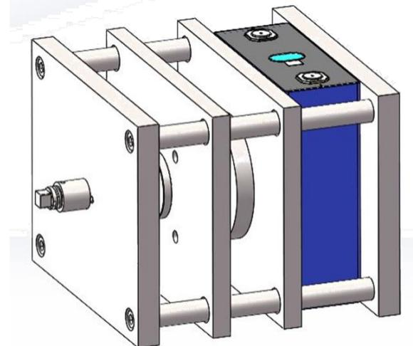
Fig. 5 Diagram of cell with swelling force clamp
