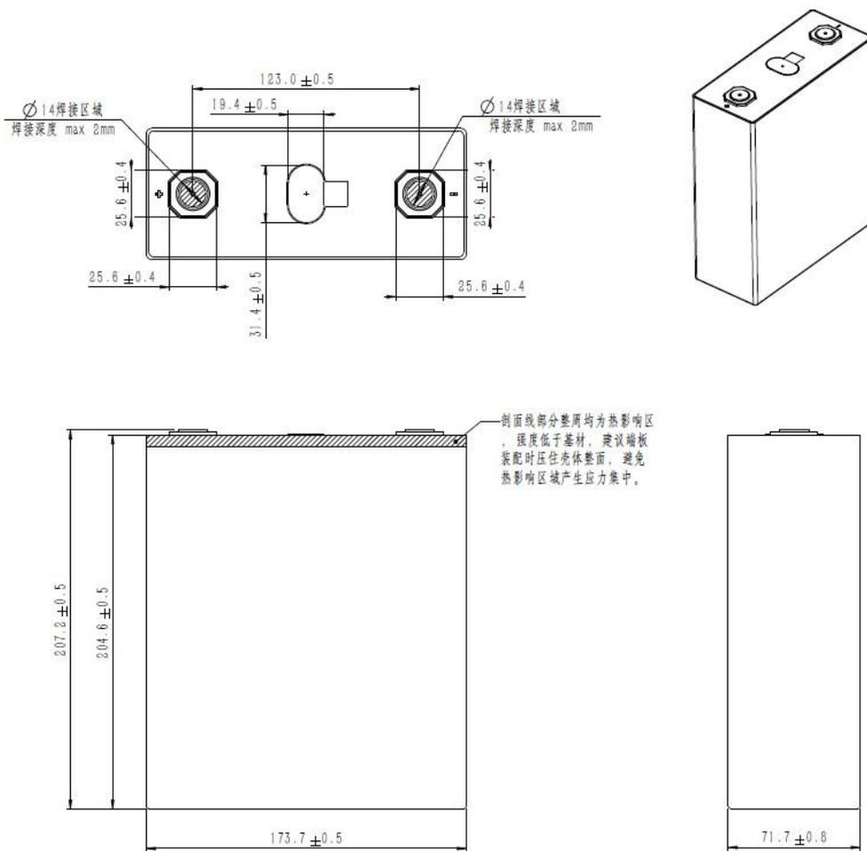
Fig. 15 Diagram of cell size and appearance
