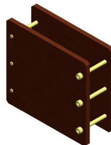
Fig. 2 Diagram of the clamp covered with insulation film
