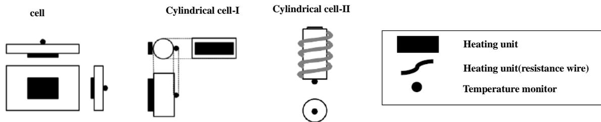
Fig. 7 Diagram of thermal runaway test
