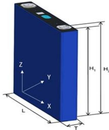
Fig.6 Diagram of LF150Cell direction
